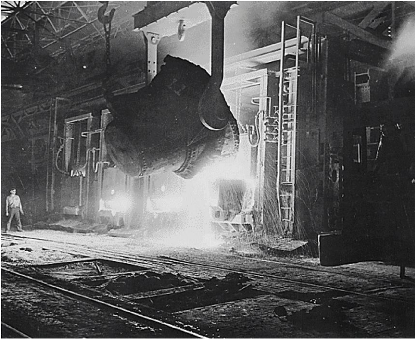
A “steel pig” pouring molten steel into a mold. Jones & Laughlin Steel Company, Pittsburgh, PA, 1942. U.S. National Archives and Records Administration.
